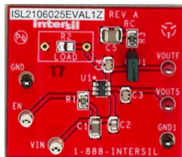
FIGURE 1. VOLTAGE REFERENCE EVALUATION BOARD
